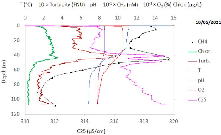
Figure 2: CH<sub>4</sub>, chlorophyll, turbidity, temperature, pH, oxygen and conductivity (C25) profiles at LéXPLORE station on 10/05/2021.
