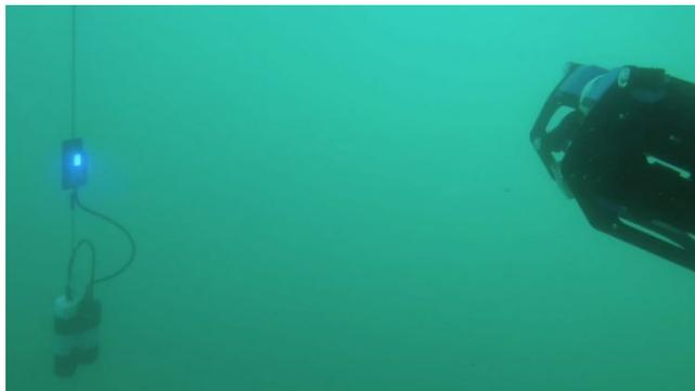
Figure 1: BlueROV with LUMA modem (right) downloading data from logger (left)
