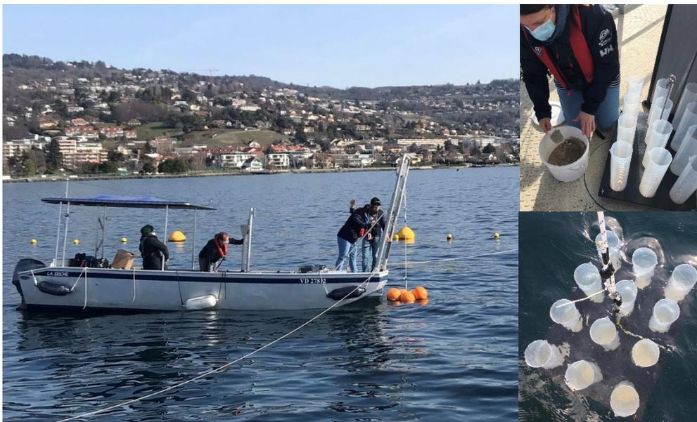
Filling the tubes with a bottom of clean sand before the ExpoSET systems disappear for 4 months at a depth of 30 m depth in the LéXPLORE protection perimeter
