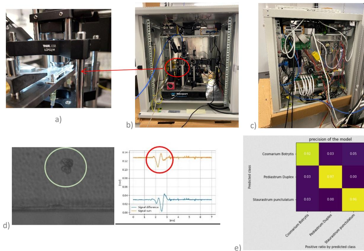
Figure. (a) Close-up view of the glass biochip with the microscope and waveguide on the side. (b) fully autonomous instrument front view and (c) rear view (shown in open-configuration). The automat handling the fluidic processing is embedded in the instrument. (d) Example of wavelet acquired for one type of algae. (e) Training algorithm, showing the accuracy of the detection achieved for three species mixed randomly (specimens provided by EAWAG).
