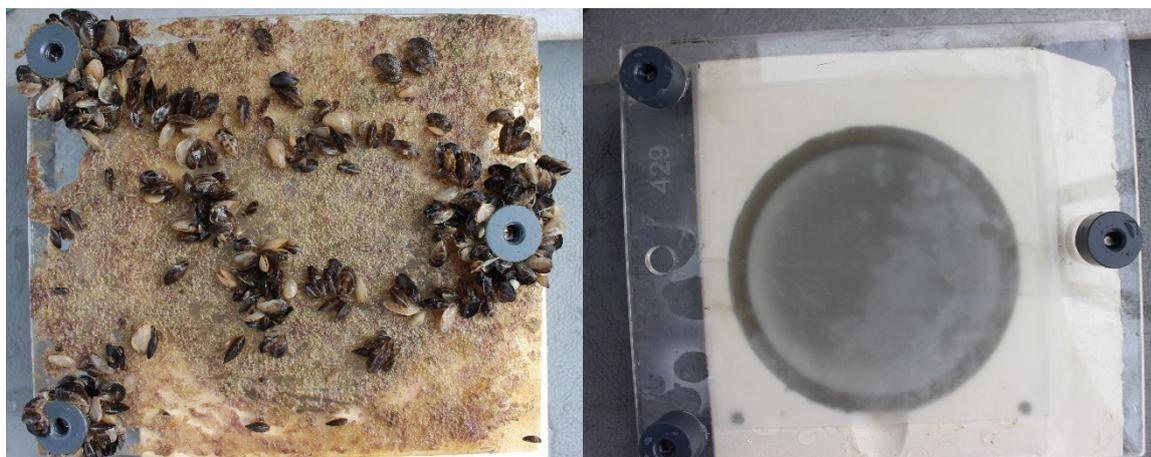
Figure 1: shows the colonisation between June and September 2020. The left panel shows a plate from 9m depth including a lot of quagga mussels and biofilm. On the right, the plates is retrieved from 60m and does not show any visible biofilm nor mussel settlement.
