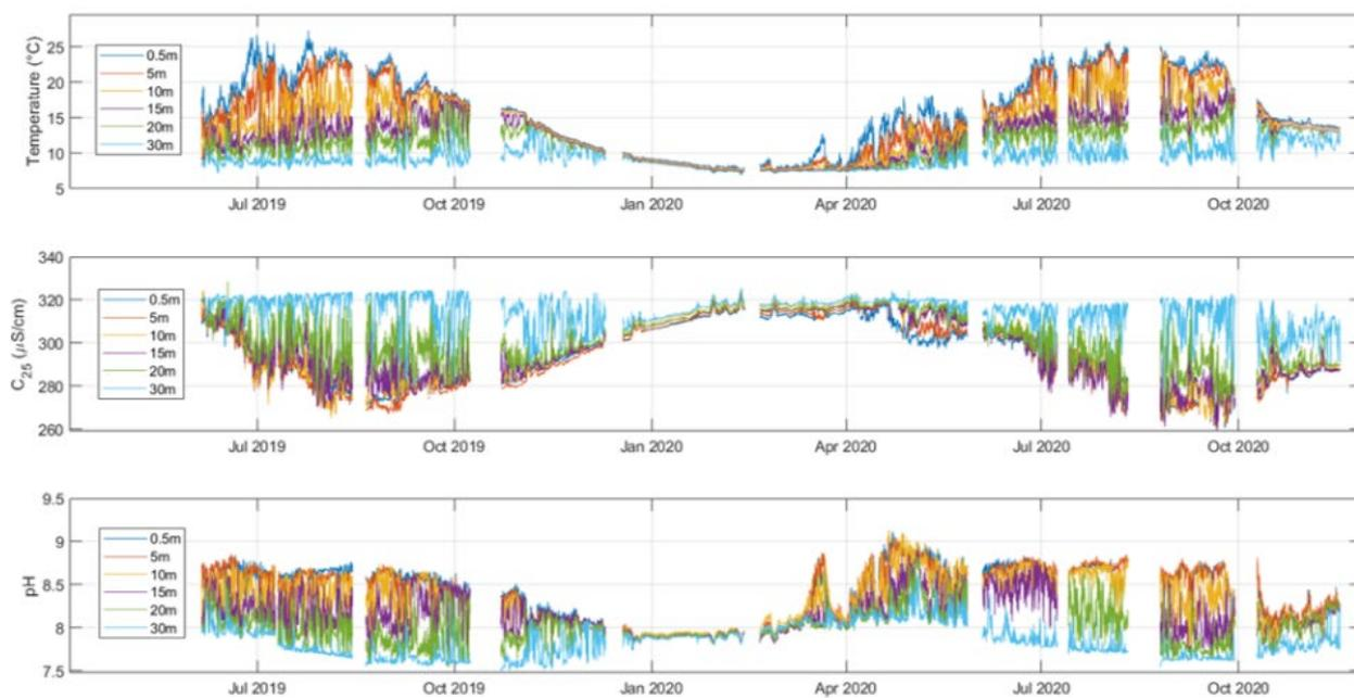
Figure 1: Timeseries of Temperature, Specific conductance ( $C_{25}$ ) and pH measured at LéXPLORE since June 2019, and below correlations with  $Ca^{2+}$  and TA concentrations.
