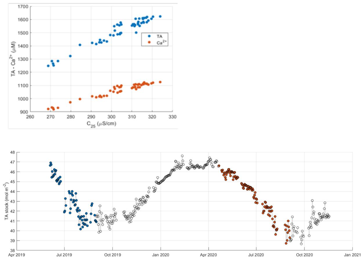
Figure 2. Daily stock of TA integrated between 0 and 30 m depth and specific periods of depletion in blue (2019) or red (2020) corresponding to calcite precipitation.
