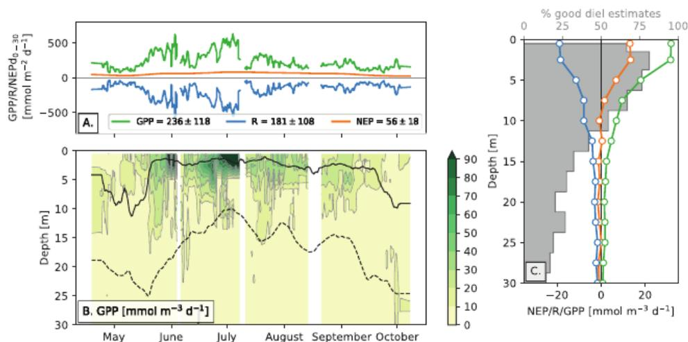
Figure 1: Primary and net ecosystem production estimates over summer 2019 derived from the diel DO method using in-situ data of moored instruments at the LéXPLORE platform.
