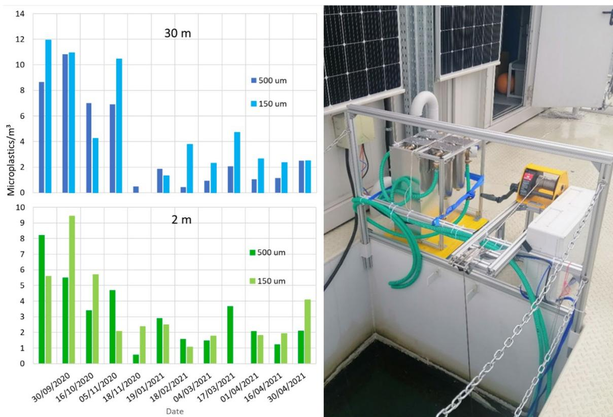
Figure 1: a. Total Microplastics/ $\text{m}^3$  in pumped water separated by depth. b. The pump apparatus on LeXPLORE.
