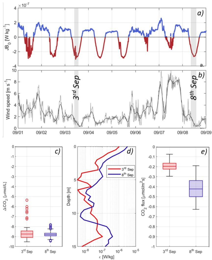
Figure 1: The effect of residual currents on air-water  $\text{CO}_2$  fluxes. Besides similar concurrent weather conditions (a-b) and air-water  $\text{CO}_2$  gradients (c), the effect of an antecedent strong wind event determines larger turbulence on the 8<sup>th</sup> than on the 3<sup>rd</sup> of September 2020 (d) thus resulting in larger air-water  $\text{CO}_2$  fluxes (e).
