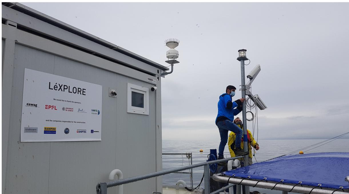
*Photo of the radiometers installed on LéXPLORE*
