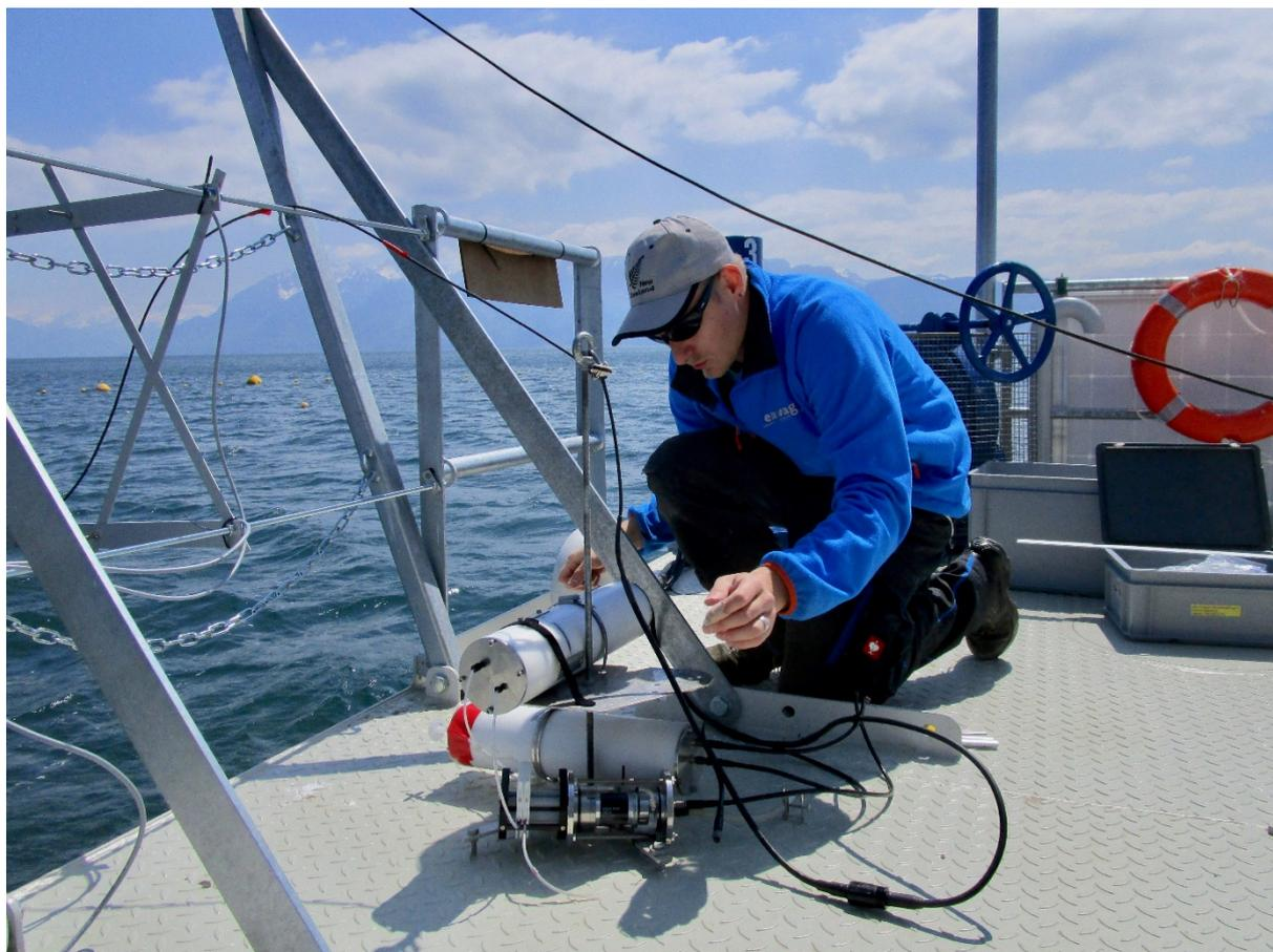
*Deployment of the micro-Titrator on LéXPLORE platform*
