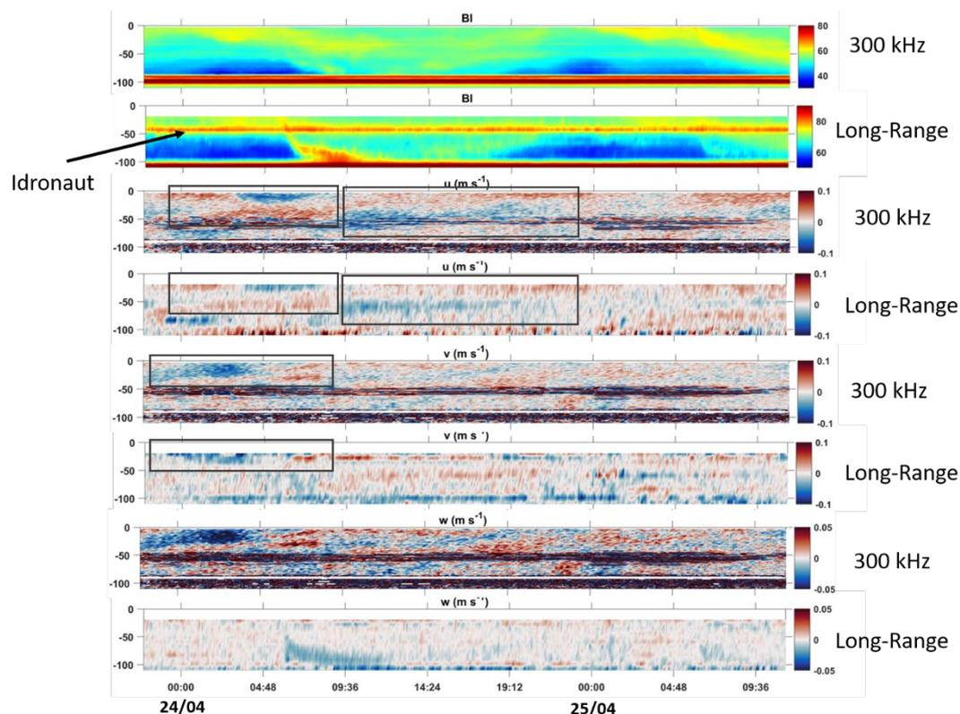
Figure 1: Backscattering (in dB) and east ( $u$ ), north ( $v$ ) and vertical ( $w$ ) velocities (in  $m s^{-1}$ ) measured by the 300 kHz ADCP and by the Long-Range ADCP (150 kHz) from 24th April to 25th April 2021.
