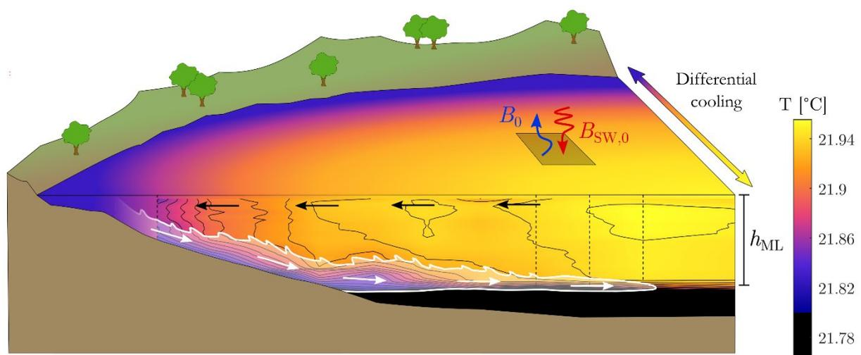
Figure 1 – Schematic of the thermal siphon induced by differential cooling. The density current and the surface return flow are depicted by white and black arrows, respectively.
