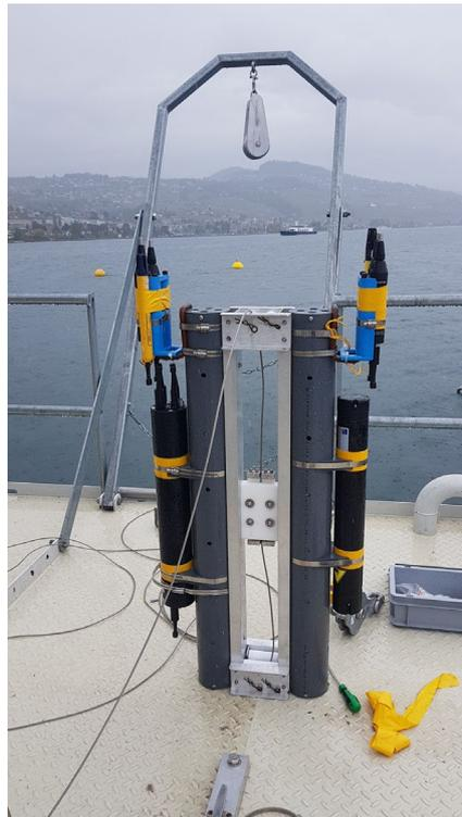
*Photo of the autonomous turbulence profiler used on the LéXPLORE platform*
