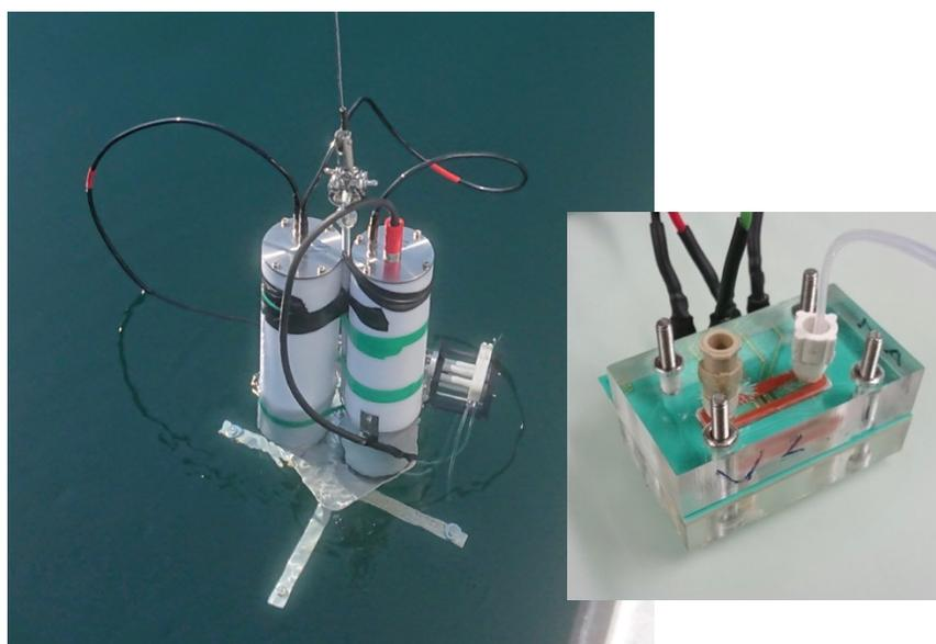
*Micro-Titrator for in-situ Alkalinity measurements, with titration cell.*
