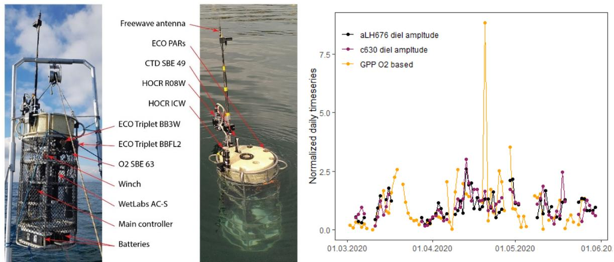
*Figure 2: Left and central panels: detailed view of the WetLabs Thetis profiler operated from the LéXPLORE platform. Right panel: timeseries of aLH676, c630 and O<sub>2</sub>-based GPP estimates during the period March-May 2020, normalized by the overall observed average values. After Minaudo et al., under review in *Environmental Science & Technology*.*
