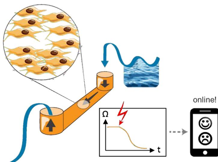
*Working principle of the RAINBOW<sub>FLOW</sub> CHIP<sub>ONLINE</sub> biosensor for water quality monitoring: fish cells are exposed to water from Lake Geneva and cell viability is measured continuously, data are available online in real-time.*
