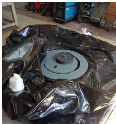
Fig. 1. Middle panel: CAD drawing showing cross-section of the EC with the optical module of ANTARES contained in a light-tight tarpaulin. Bottom panel shows the EC assembled at EPFL in the course of the first year of the project. The EC will be suspended under a floating platform (shown in the top panel, already at EPFL) carrying a hut with power supply and readout electronics modules, with a solar panel on its roof (still “to do”).
