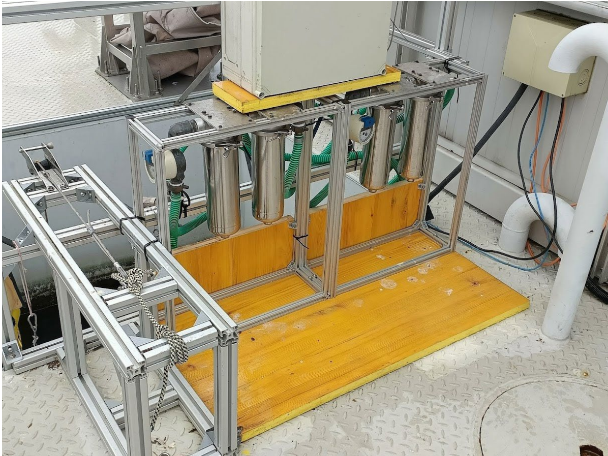
Figure: Optimized microplastics sampling system used on LéXPLORE
