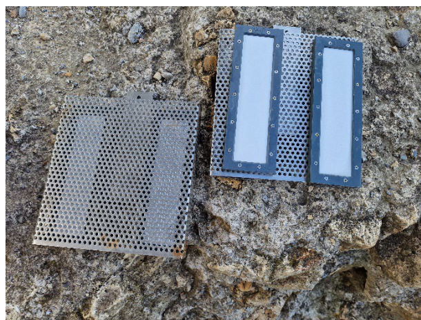
Figure: DGT samplers consist of a plastic housing containing a plate with a diffusive gel that allows only labile species to reach the underlying binding resin.
