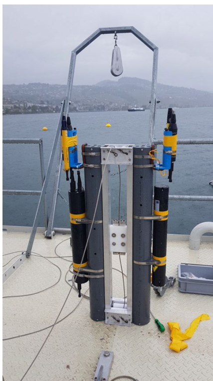
Figure 1: Photo of the autonomous turbulence profiler used on the LéXPLORE platform
